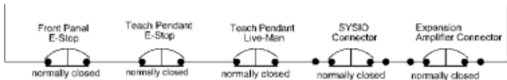
Figure 14: The E-Stop circuit showing all possible E-Stops installed and operational.
