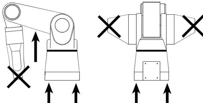
Figure 9: Always grasp the robot under the base or arm link.
