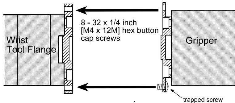
Figure 33: Attaching the wrist tool flange and gripper adapter plates together
