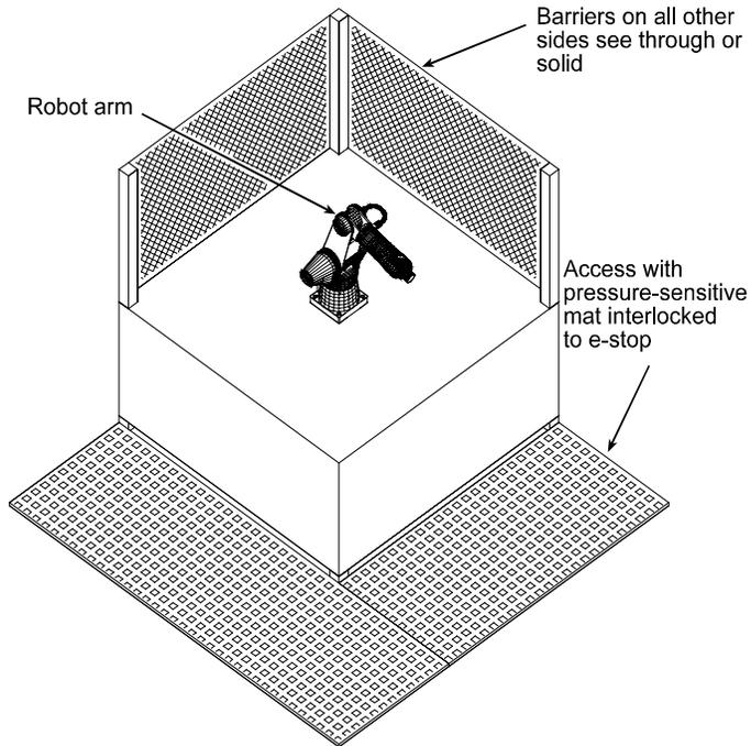
Figure 14: Example of barriers and interlocked pressure mats.
