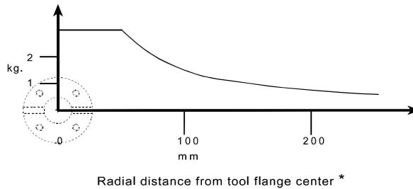
\* Maximum payload is the lower of axial and radial
