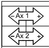
Figure 29: Teach pendant axis keys. In limp mode, a positive (+) key limps a joint and the negative (-) axis key unlimps the joint. “Ax 1” for axis 1 (the waist joint), “Ax2” for axis 2 (the shoulder joint), etc.
