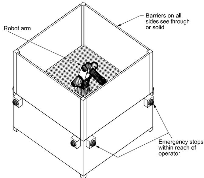
Figure 15: Typical barriers and remote E-Stop buttons.
