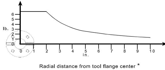
\* Maximum payload is the lower of axial and radial
