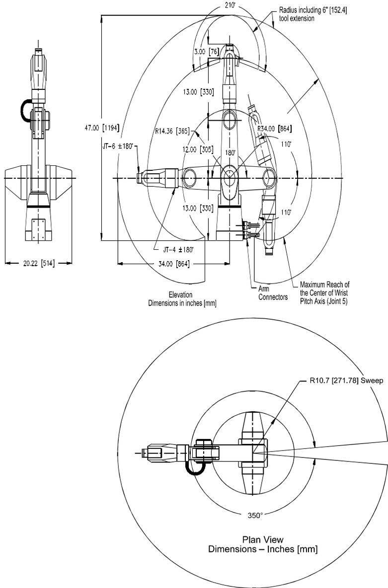
Figure 2: Range of motion and the dimensions of the sections of the A465 arm.
