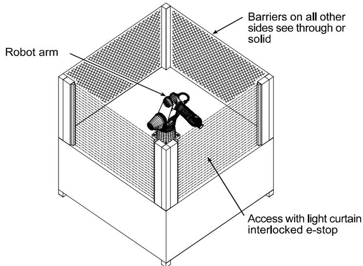
Figure 12: Example of barriers and interlocked light curtain.
