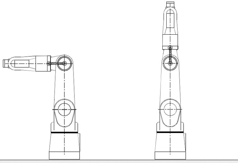
Figure 23: Safe starting positions for homing.
