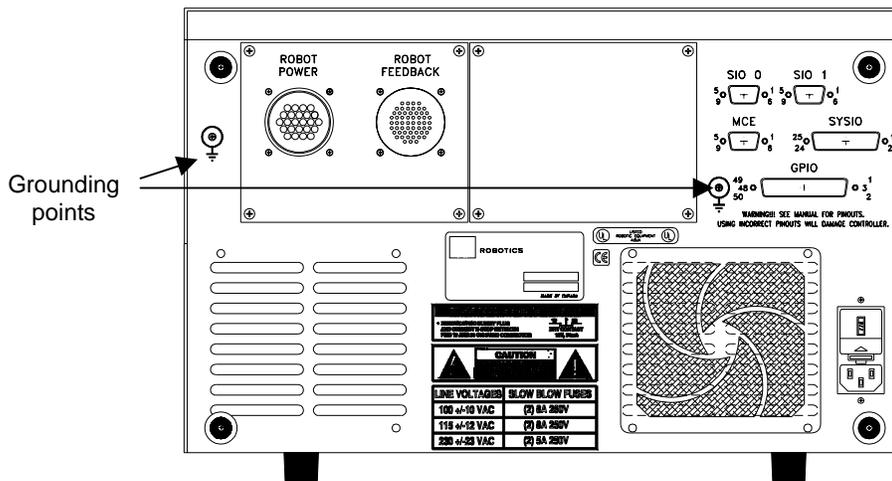
Figure 21: Controller rear panel for the C500C controller
