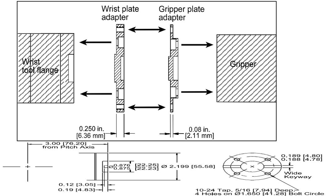
Figure 30: Mounting dimensions of the tool flange for the gripper in inches [mm].
