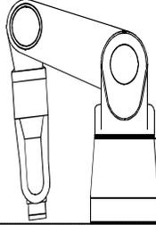
Figure 22: A465 arm shipping position. This is not a safe starting position.
